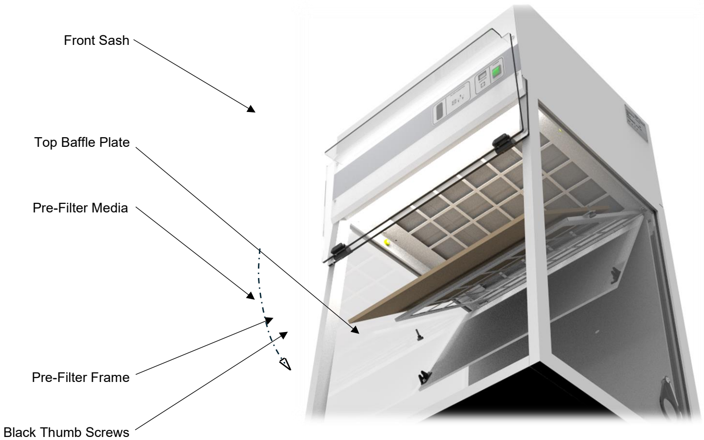
Figure 4 Pre-Filter Removal / Installation
