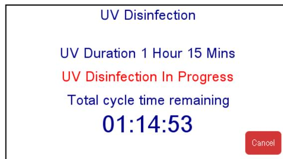
If the safety screen is removed or the "cancel" button is pressed the cycle will terminate.
