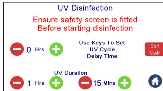
The safety screen is interlocked with the UV disinfection cycle and the cycle will not run if it is not fitted. Use the arrow keys to set the disinfection time and cycle start delay if required.
