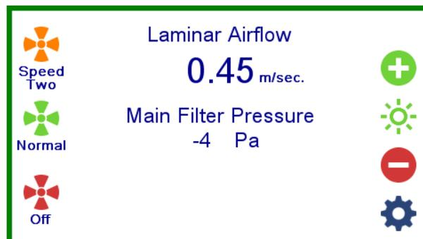
SPEED 2 is a preset that can be set higher or lower than NORMAL. An example of its use could be to set higher to rapidly purge the cabinet\*\* or lower to conserve energy when a non-critical task takes place within the cabinet.
