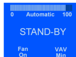
VAV Min Reduced velocity: Damper closes to reduce airflow - sometime required for powder work
