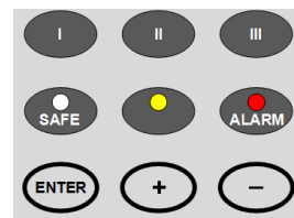
Sash above maximum working height with low airflow Both the amber & red LEDs will illuminate
