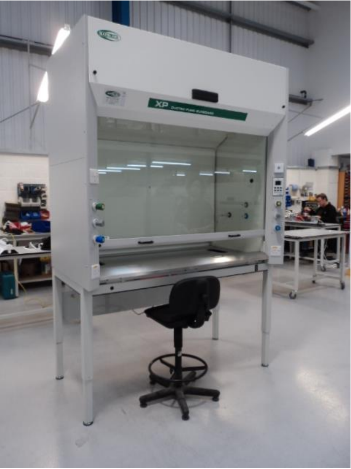
Airone XP: 54 VAV units, 4 with DDA compliant adjustable height stands
